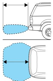
The reverse sensing system is automatically enabled when the gear selector is placed in R (Reverse) and the ignition is ON. A reverse sensing control allows the driver to disable the reverse sensing system only when the ignition is ON, and the gear selector is in R (Reverse).
